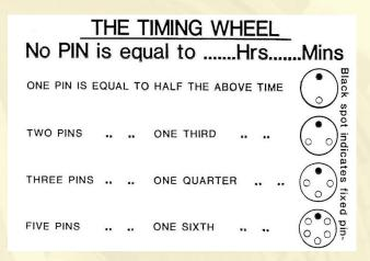
The black dot indicates the fixed pin (ie the small raised line on the timing wheel) and the white dots indicate the <u>pin positions</u> (NB with no pin(s) inserted there are seven available pin holes in the timing wheel). It should be noted that the position of the fixed pin will depend upon where the timing wheel is in the timing cycle; consequently it may not be situated at 12 o'clock as per the diagram.
