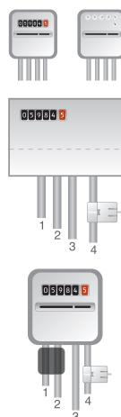
Dual Tariff meters will often have an Auxiliary cable running between Cable 3 and Cable 4. Auxiliary cables will be smaller in diameter than the feed cables, and will run into an adjoining metering device.
