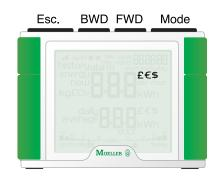
Default cost is 11p/kWh. This is the average price per kWh electricity companies charge. Use **BWD** and **FWD** to change the cost per kWh. Press **Mode Button** to save your setting. Voltage setting will flash.
