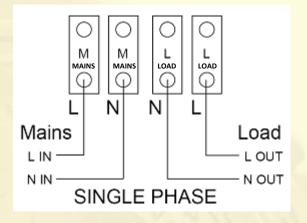
As you look at the terminal block the two left hand terminals are live and neutral and the two right hand terminals are neutral and live is common neutral on the middle two terminals.
