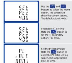
The PT Rate is the PT Primary divided by the PT Secondary. For Example: Voltage Transformer - 11000 $\div$ 110=100, so the PT Rate would be 0100 and the PT2 would be 110.
