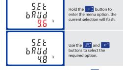
On completion of the entry procedure, hold the E button to confirm the setting.
