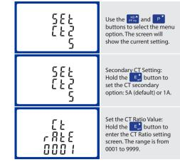
Example: 200/5A Current Transformers - 200÷5=40, so the CT Rate would be 0040 and the CT2 would be 5. On the MID Version, you can only program the
