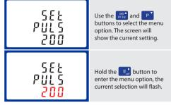
Use the weights and P buttons to choose the desired pulse rate. To save the new setting, hold the E, button for 3 seconds until the selection stops flashing.
